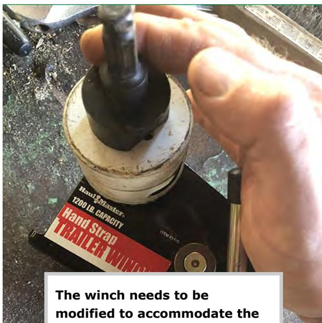
**The winch needs to be modified to accommodate the tarp roller by cutting part of the bracket out.**
