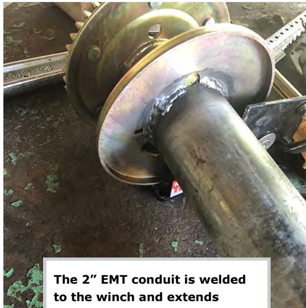
**The 2" EMT conduit is welded to the winch and extends through the bracket to form the mechanism to roll the tarp.**
